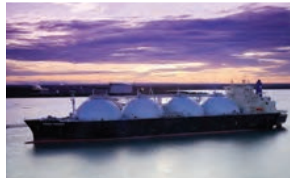
The LNG tanker Energy Advance departs Darwin with a cargo destined for Japan. LNG is transported via double-hulled tankers which are specially designed and insulated to prevent leakage or rupture. Once it reaches its destination, LNG is pumped from the storage tank and heated to convert it back into natural gas.
